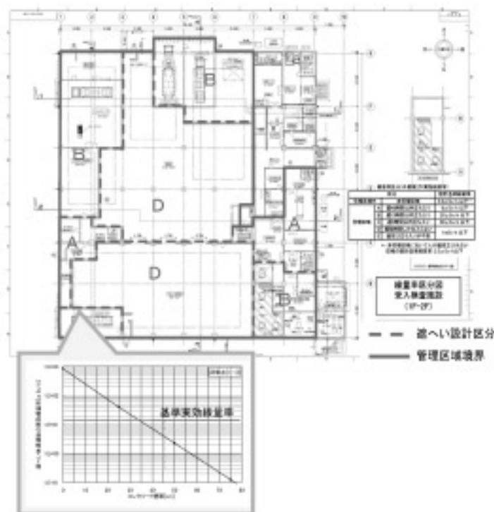
Fig.5 Outline of shielding calculation for the waste package reception and inspection facility
